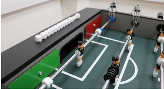
Figure 2: The goal of the haptically augmented foosball. On the side of the goal, it is possible to see the sensorized plates. Hitting the red plate blocks the opponents' rods, hitting the green plate releases the friction previously applied on one's own team.
